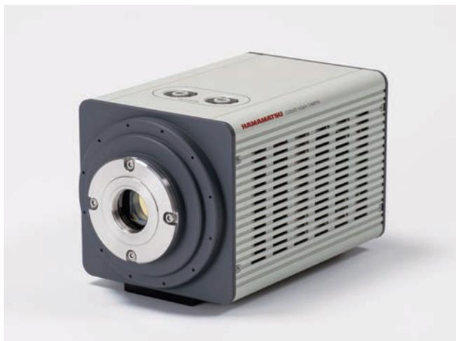
The C12741-11 is a near-infrared camera which employs a 640 pixels × 512 pixels InGaAs sensor. -70 °C peltier cooling significantly reduces dark current which leads to improved image quality and allows imaging with long exposure time.
