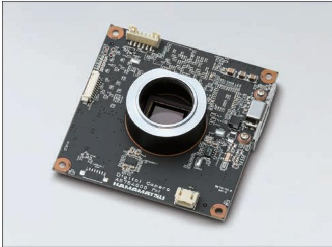
The core of the C13949-50U camera is the scientific image sensor, an advanced CMOS detector that simultaneously achieves high resolution, fast readout speeds and low noise. With its small size, board-level design and simple, low-cost integration using USB 3.0, the C13949-50U is the ideal camera for OEM scientific imaging.
