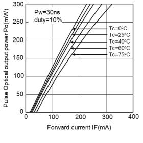
Pulse Optical Output Power vs. Forward Current
